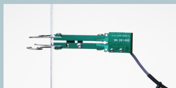
Model 3442 with 6.0 mm gauge length and \pm 5.0 mm/ \pm 1.0 mm ( \pm 83\% /-17% strain) measuring range
