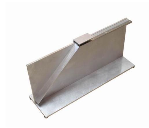
The Cantilever Bend Test is a very simple test used to find the bend length and calculate the flexural rigidity of fabrics. The fixture has a numbered scale to measure the correct bend length. The bend angle is set to 41.5 degrees but it can also be made to 45 degrees.
