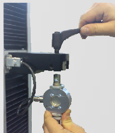
Easy load cell exchange
