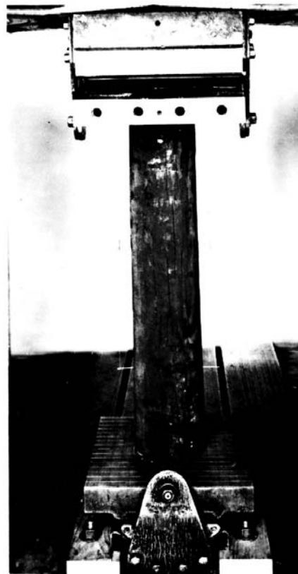
FIG. 5 Example Test Setup for a Short Specimen Compression Parallel to Grain Test (Two Bearing Blocks Illustrated)
