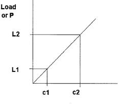
**Compliance Correction for Displacement (D) or Strain**
