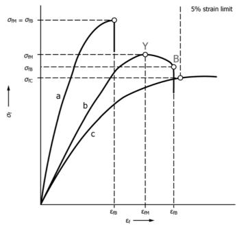
Note 1—Curve a: Specimen that breaks before yielding. Curve b: Specimen that yields and then breaks before the 5 % strain limit.
