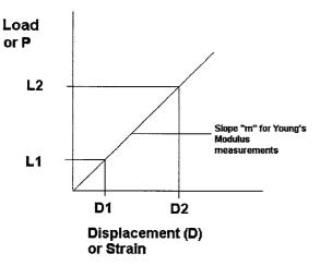
FIG. X1.1 Example of Modulus Curve for a Material
