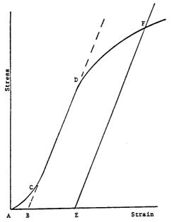
Note 1—Some chart recorders plot the mirror image of this graph. FIG. A1.1 Material with Hookean Region
