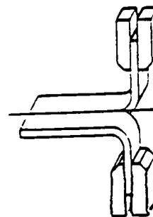
Positioning of trouser test piece in testing machine
