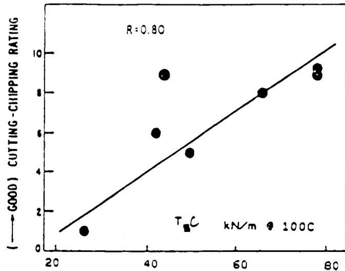
FIG. X1.3 Tear Strength (CP-Specimen)  $T_c$  versus Cutting-Chipping Performance
