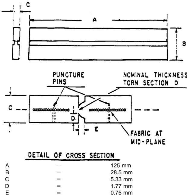
FIG. X1.2 Schematic Diagram of "Constrained Path" Tear Test Specimen
