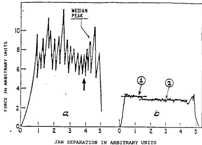
NOTE 1—Curve a—peak or knotty tear Curve b—smooth tear
